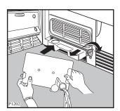
The reservoir must be re-inserted correctly.
